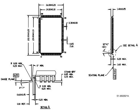
DIMENSIONS ARE IN MILLIMETERS.
